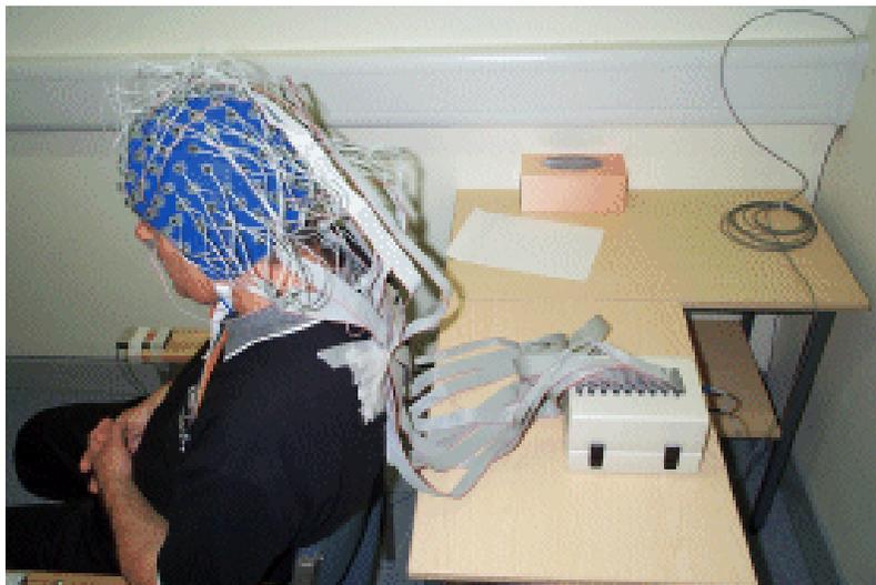
Figure 1. The BioSemi system in working setup
